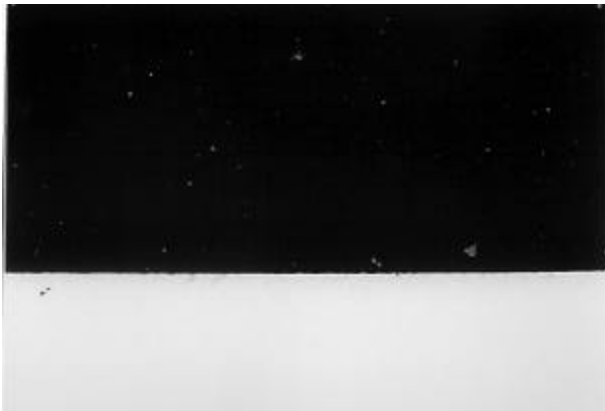
Figure 5: Typical polished microstructure of the wrought Alloy 49 Glass Seal. The glass is the dark area and the white area is the metal. 250X magnification.
